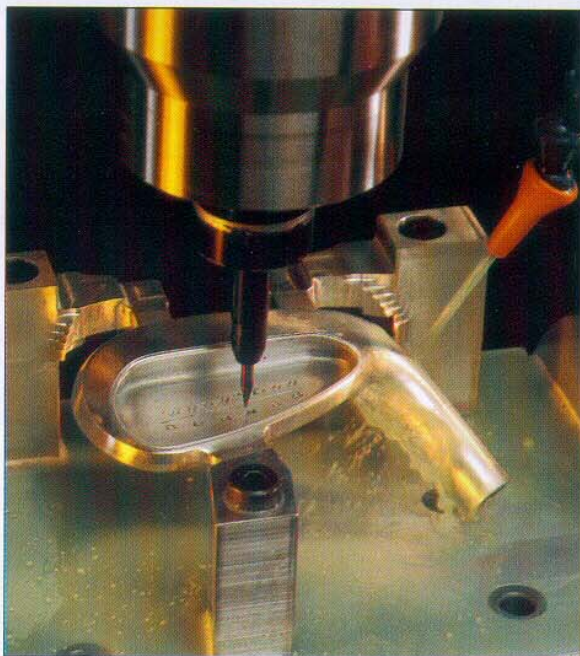
Engraving a master model for a new club head is done on a Haas VMC with IBAG's "Plug and Go" spindle.
