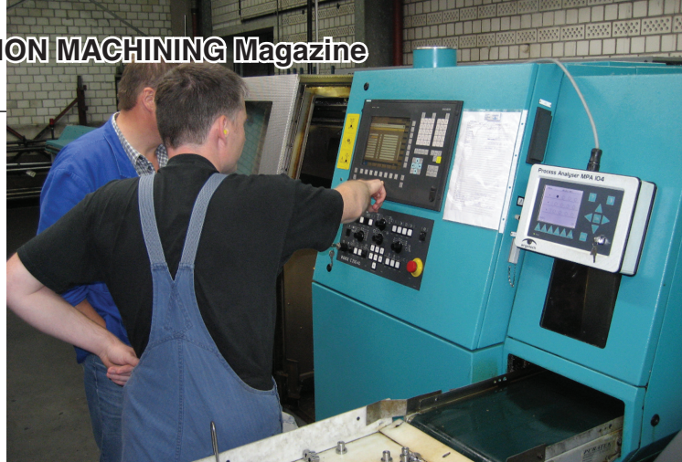
▲ This process monitor on a CNC machine measures the machining process real-time via sensors on the machine.
