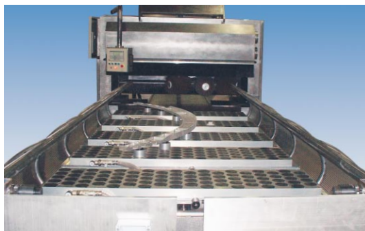
FLIP-POD™-clamping system for a CNC deburring machine, used on aeroplane parts
