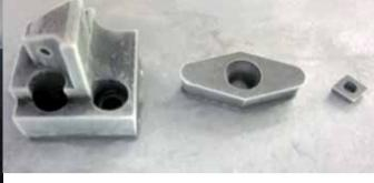
When clamping with the Ice-Vice system parts are frozen to chuck surface on a capillary film of water for machining. Even relatively uneven parts can be clamped as any gaps are filled with water. The vertical and horizontal clamping forces created are enough to hold small parts for milling, grinding, drilling or polishing.
