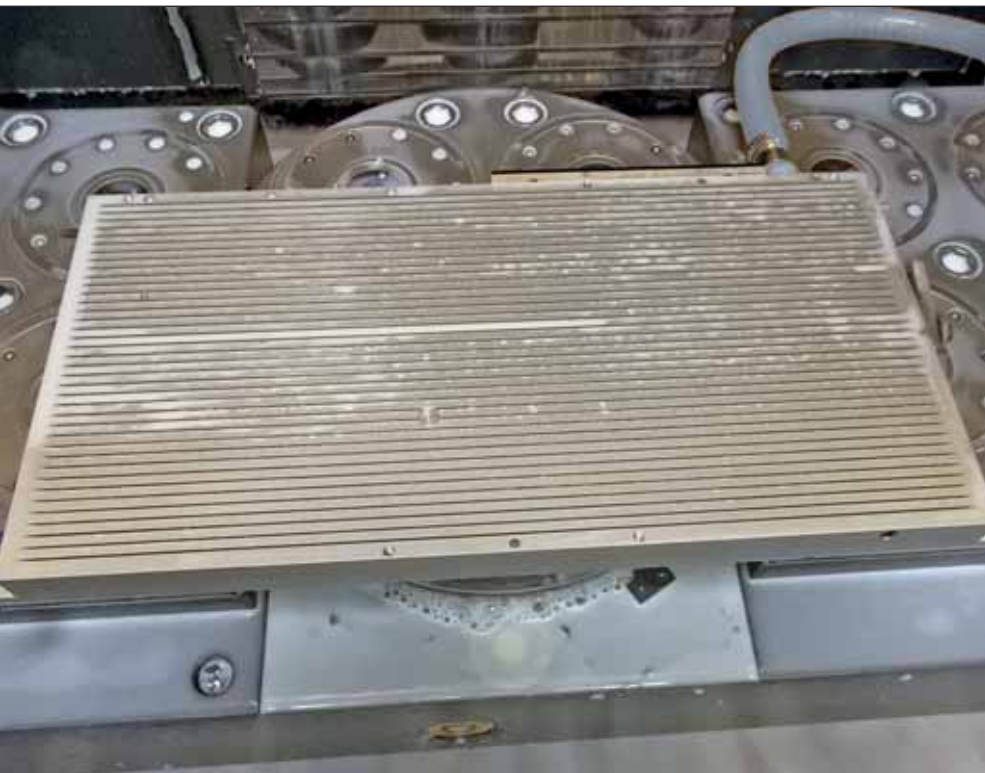
Slot vacuum chuck mounted on a zero reference clamping system
