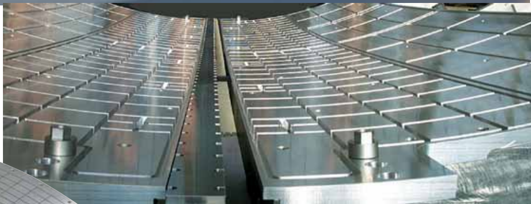
3D Vacuum chuck with several movable segments for clamping aircraft fuselage parts during milling and friction stir welding processes
