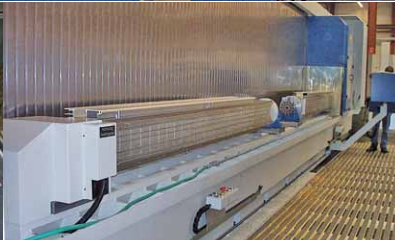
2 Rotating systems (each 3500mm) with vacuum clamping areas on all four sides for machining aluminium profiles
