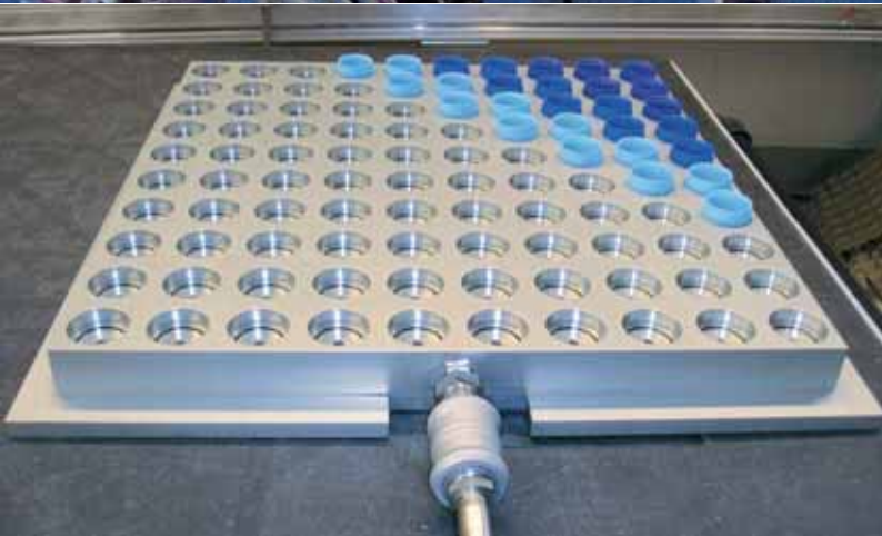
Vacuum chuck for clamping bottles tops during measuring by coordinate measuring machine
