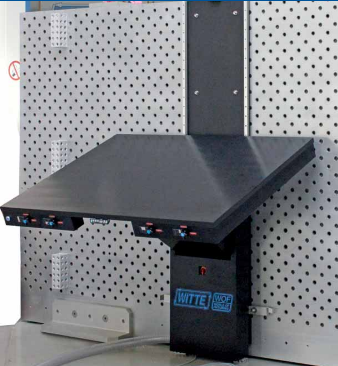
Grid hole type chuck with integrated Vilmill roller, surface area 1300x300mm
